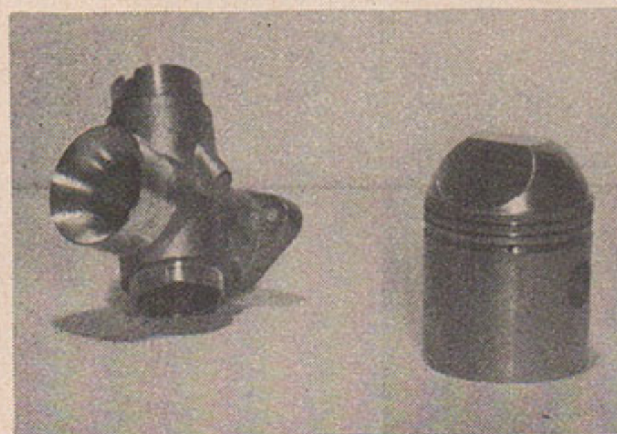
BELOW —Lewalloy Amal carburetor body and special piston, both designed for alcohol
