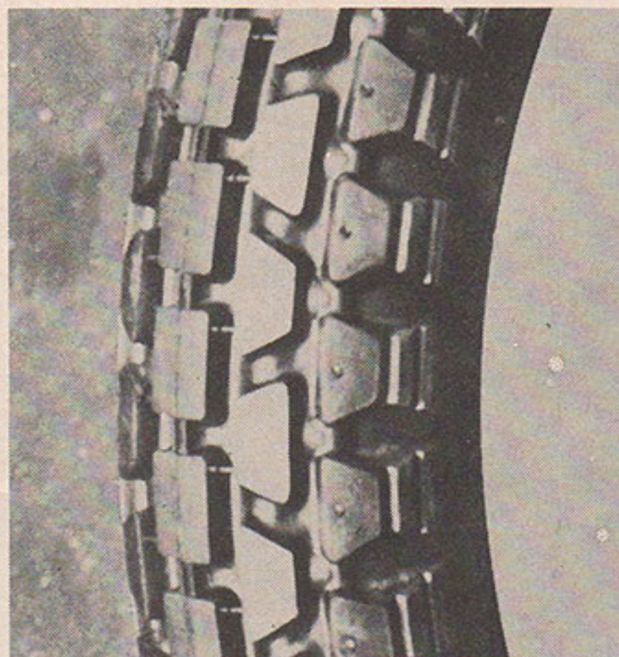
ESPECIALLY suitable for rear wheels when track conditions present "a heavy cushion" surface. Similar to track racing tire tread (shown elsewhere) but will clean better due to shape and depth of blocks on "deep cushion" surfaces
