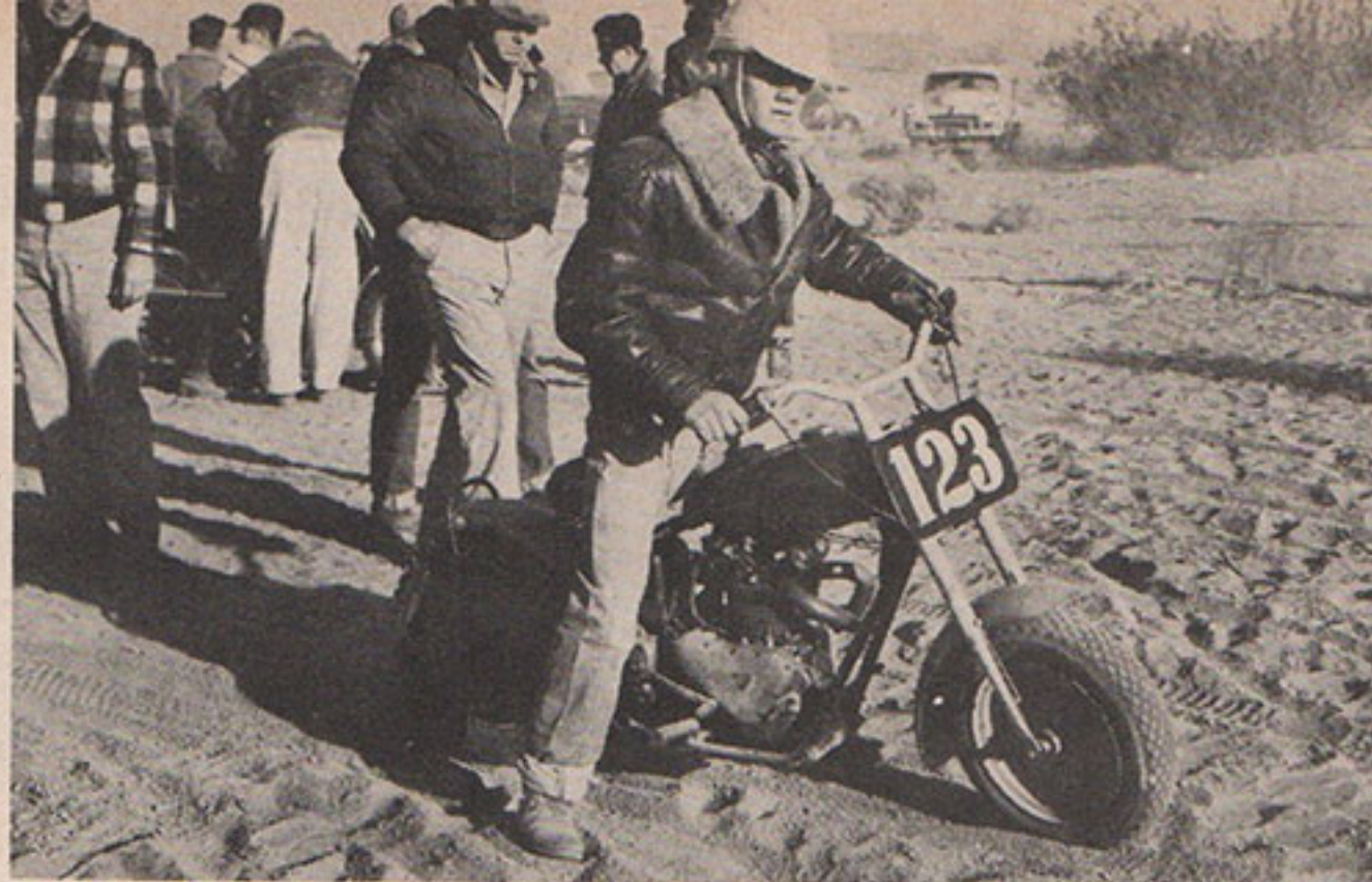
A "Mustumph"—combo Mustang frame and Triumph engine goes good
