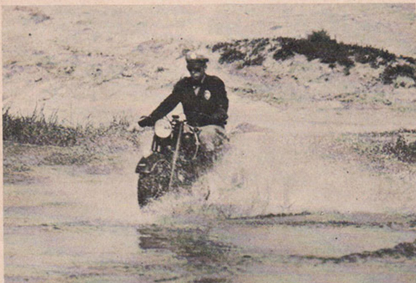
Full skirts helped, but spray from front of wheel still managed to find operator. Drip-back from front fender was practically eliminated
