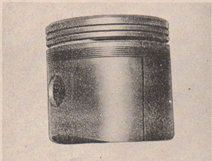
Forward side of a wire-wound AJS-Matchless piston shows "T" slot. Note five turns of wire
