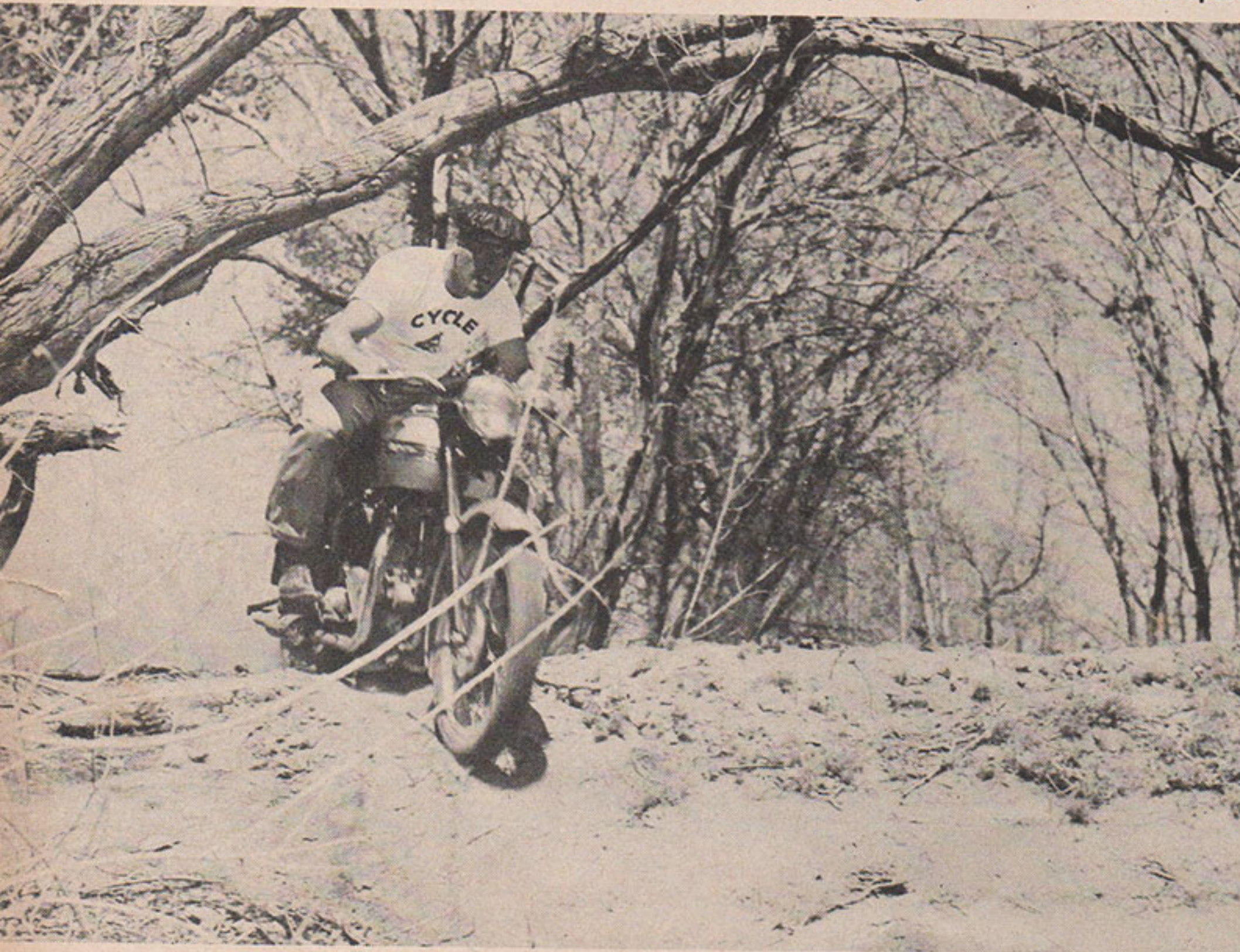
The start of an intensive four day test. Broken ground riding indicated rear spring hub needed beefing up to properly absorb 200 lb. rider when pushed hard and fast. Engine stayed very clean
