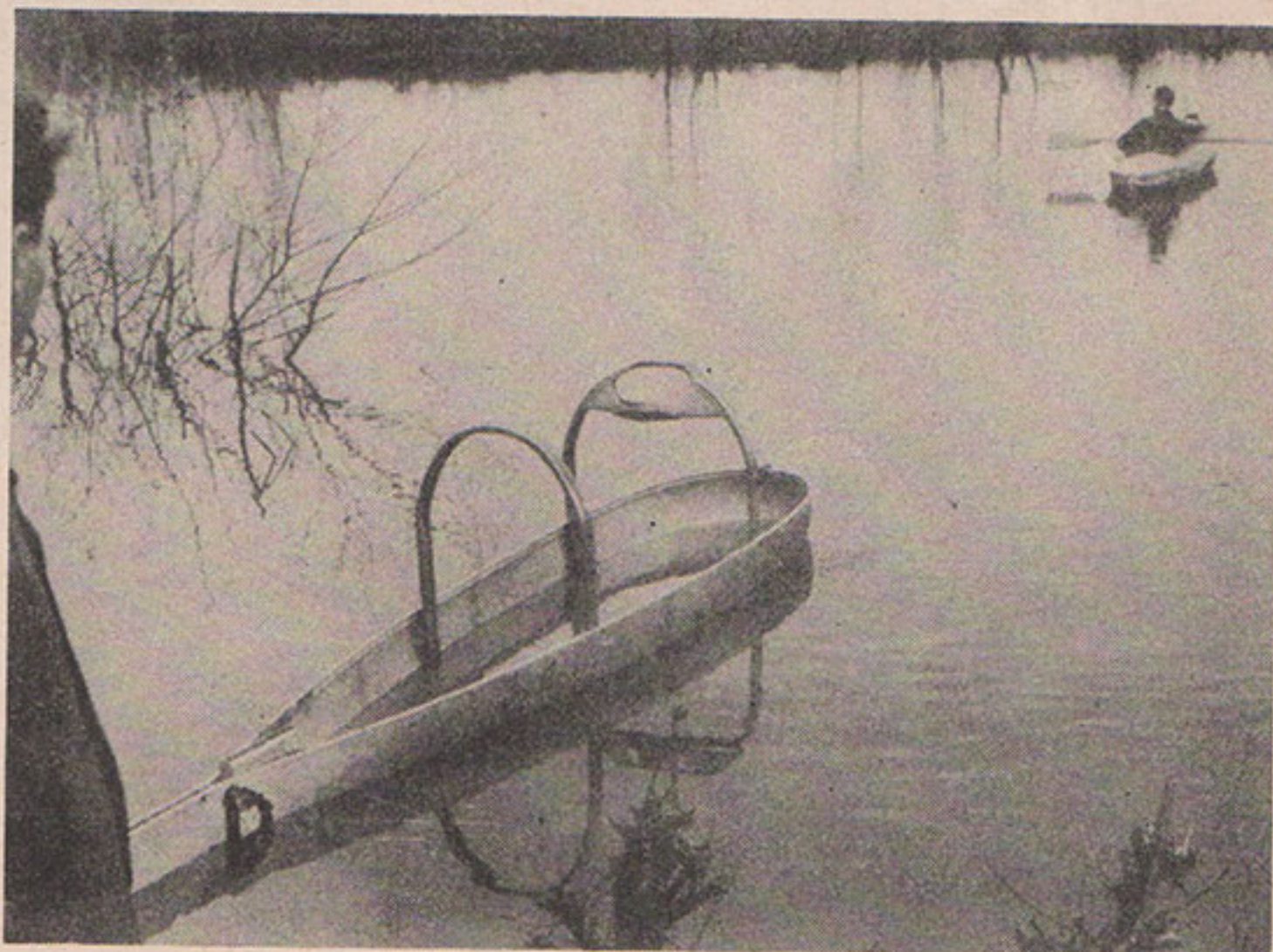
In the absence of expensive wind tunnels, an experimental shell was pulled through waters of a lake to determine proper streamlining of all-important hull. An example of infinite care to detail
