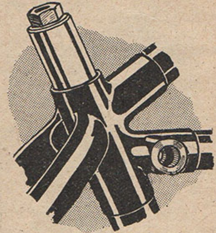
The seat lug of the 3½ h.p. Sunbeam has the rear stays brazed in. An expander bolt and cone secures the saddle-pillar.
