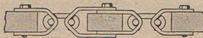
A roadside belt repair.
