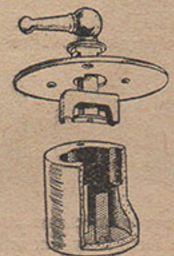
A high-tension terminal and an electrical switch made by the makers of Cooke's plugs.
