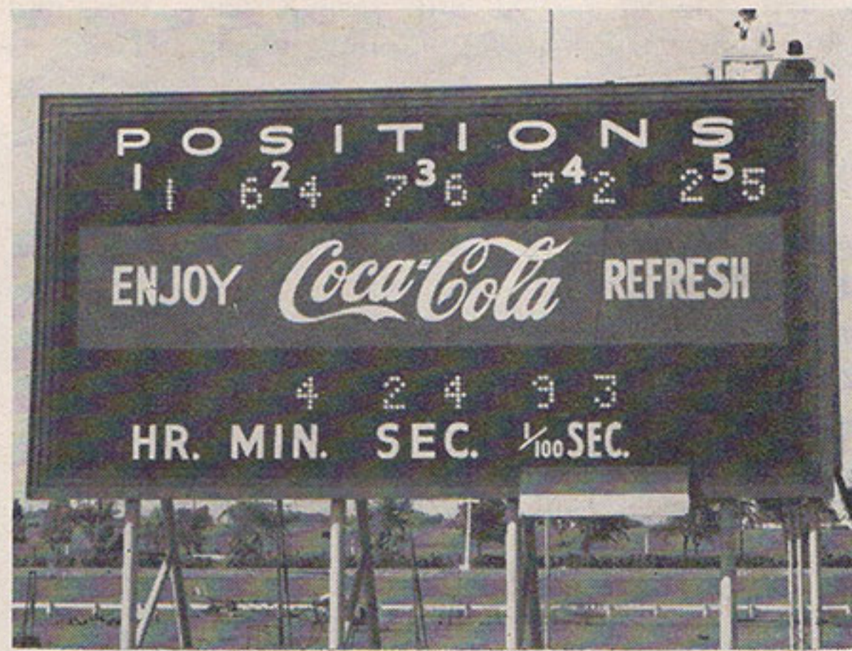
This new $10,000 scoreboard is 26 feet long, 15 feet high and reaches 32 feet into the air. Lighted numbers indicate the first five positions, number of laps completed by the leader and the total time elapsed.
