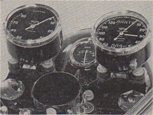
You get an 8000 r.p.m. tachometer on twin mount with precision speedometer on the Super Rocket and Gold Star Road Racer.
