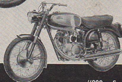
"200cc Speedster" Big brother of the 175cc; wildcat engine 25mm carb.; 63.5 bore, 62 stroke, 18 HP
