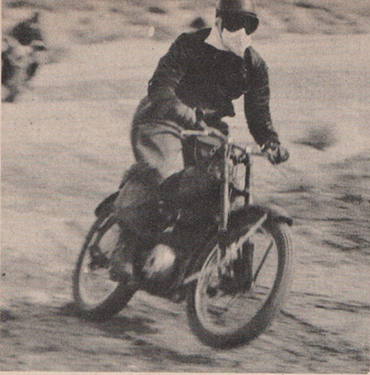
The Masked Man's two-striker rears at the first mud. About one quarter of the riders spun out at this point. Nearly all had too little clearance between the fenders and tires, mud eventually stopped wheels
