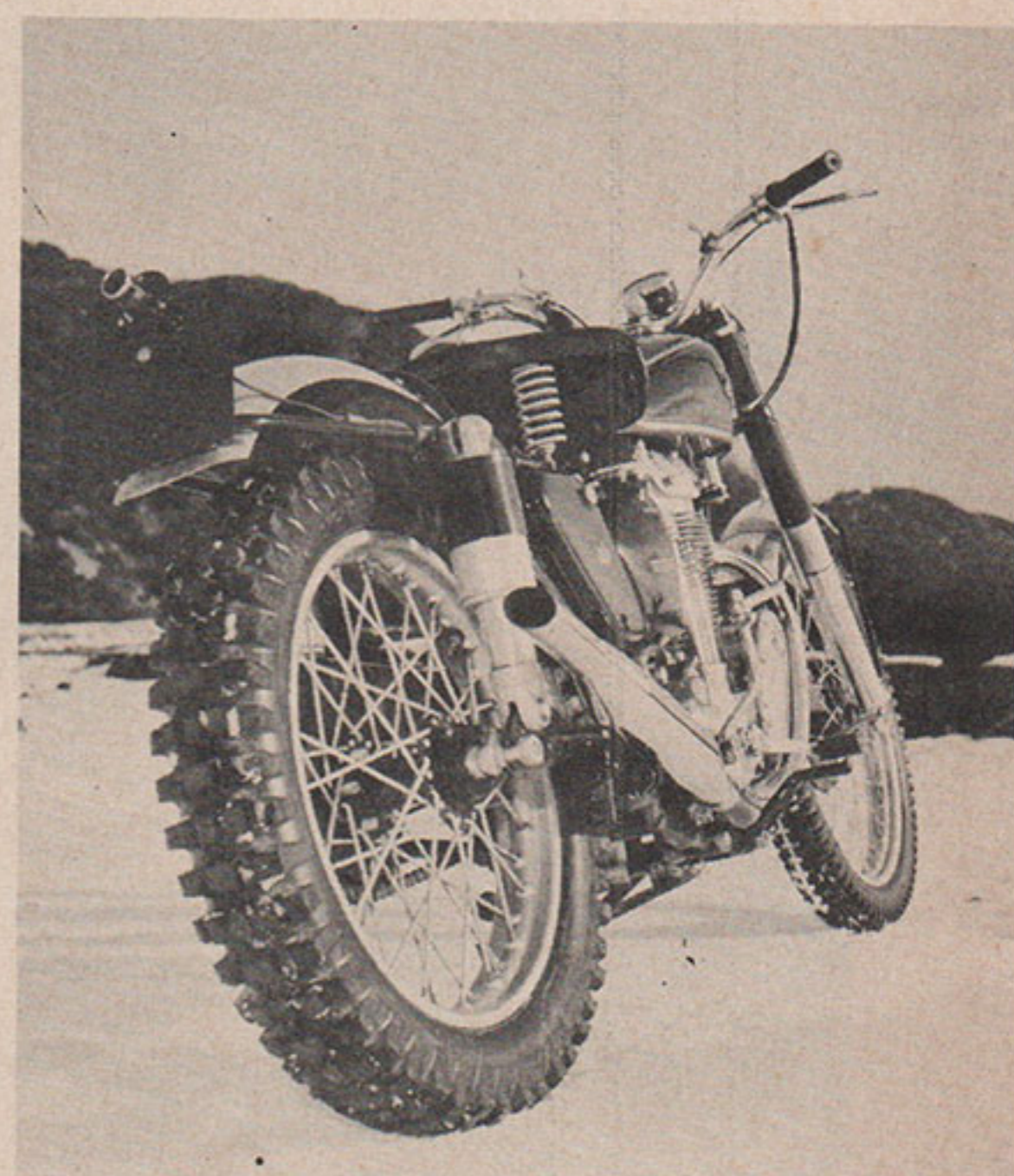
Rear wheel is practically geared to road for slogging. Fender braces are mounted outside to help keep inside of fender from loading up in mud
