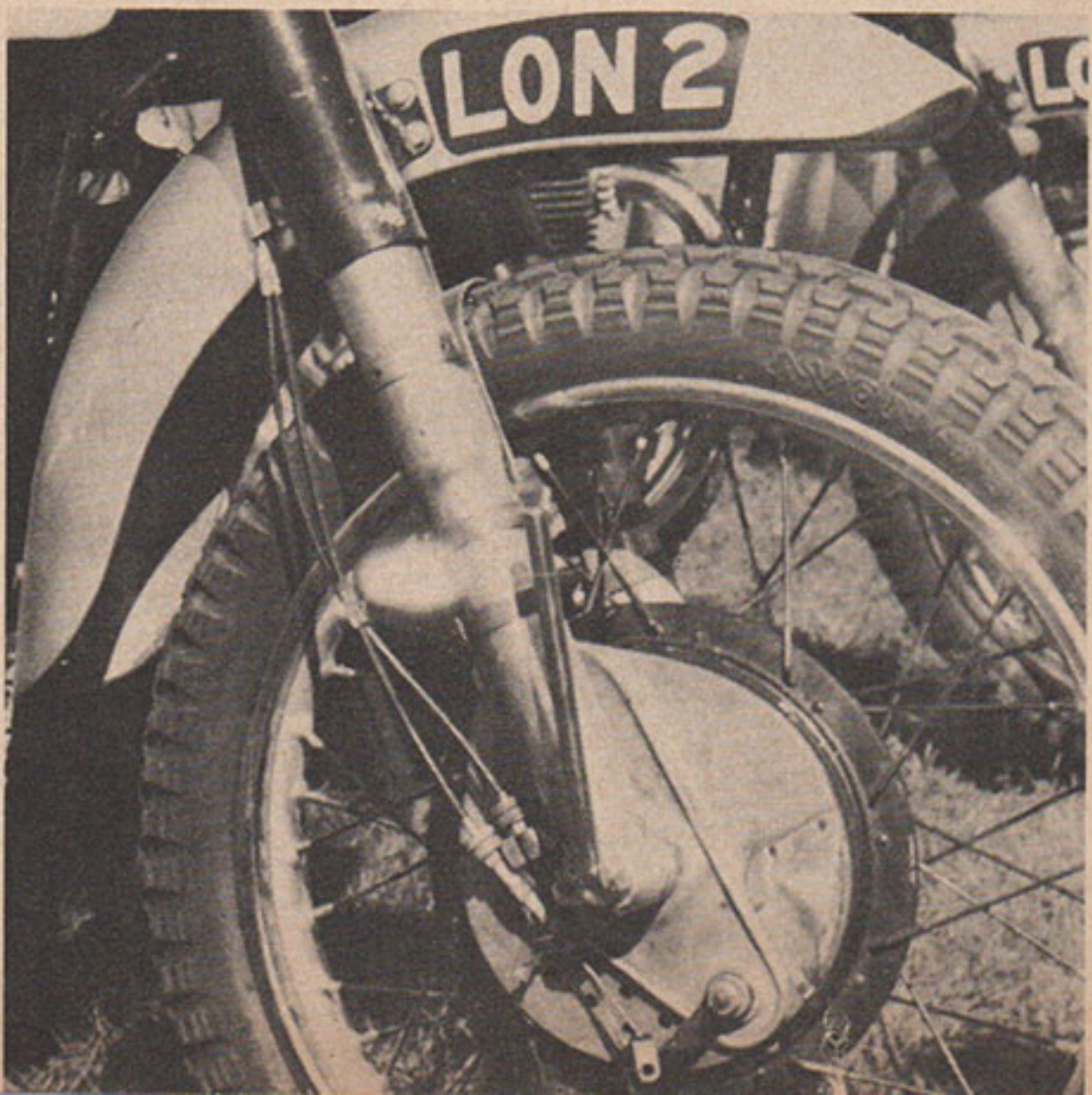
To prevent the collapse of a front wheel spring this Norton Dominator has been fortified with longer coil springs within the fork tube. In Europe the Moto Cross events compare with the American TT race, while our Hare and Hound chase is practically unheard of
