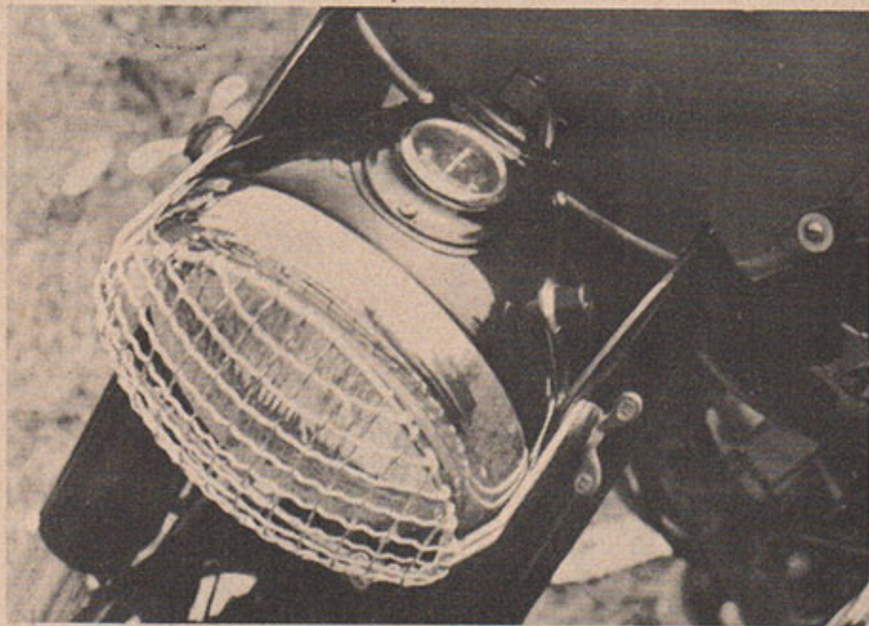
Where night riding is required in an endurance run, the loss of a headlight can cost the race or even bring disaster. This wire protective grid not only protects the lens and bulb in case of a crash, but also fends off stones thrown by wheel of man ahead
