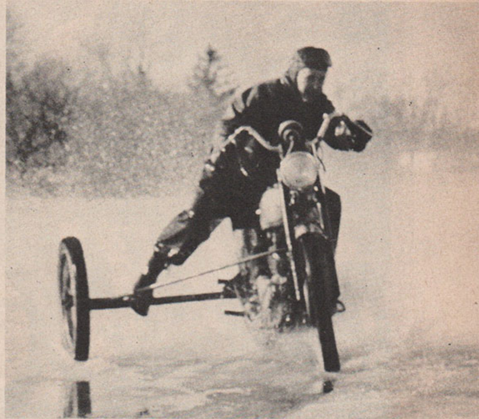
ABOVE, Elmer Brown sends up a spray negotiating a full-throttle, left turn on his Triumph Trophy model. In faster stud racing, front tires are grooved down the center to accommodate regular motorcycle chain that is secured with bolts staggered every 4 or 5 inches, assuring good steering stability. This is illustrated at left along with cross section of rear-tire studding procedure which requires that large bolts be cut through the casing, then drawn up tight with a nut on the outside. Shaded area inside tire represents protective liner to keep tube and bolt heads apart. Sketch of motorcycle shows proper linking of third wheel to frame by two pieces of tube
