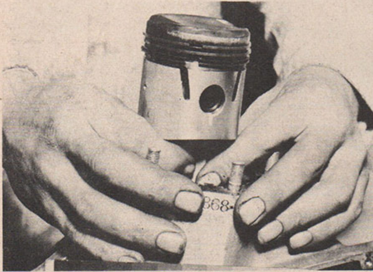
Grasp con rod firmly and exert up and down pressure. Side play is all right, but cases should be split if there is up and down play
