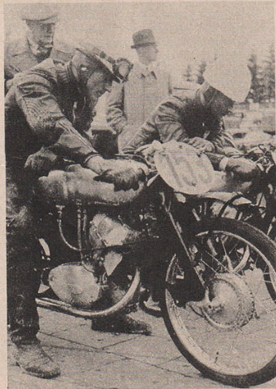
Two special NSU "Foxes" warm up at the start. Air duct reduces hot spot on right side of engine
