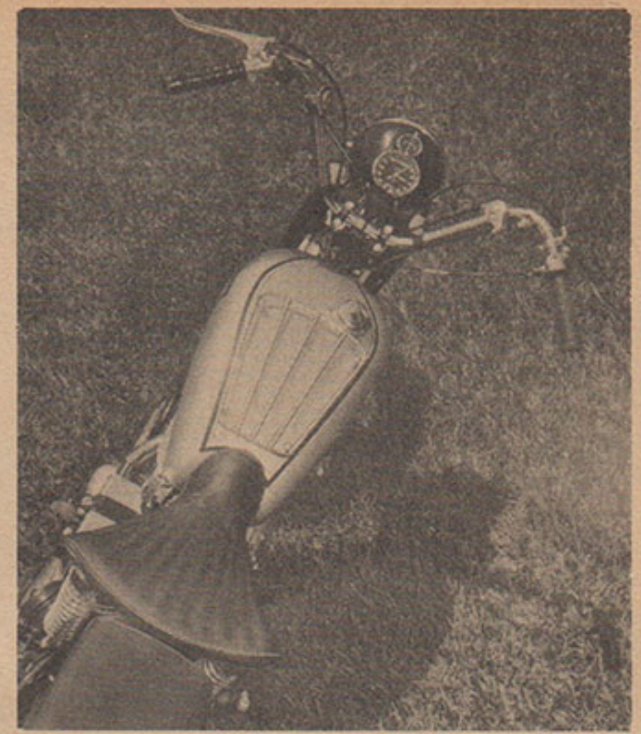
Popular narrow tank aids riding position, still holds 3.3 gallons. Parcel grid is mighty handy for strapping on jackets, maps, etc. Headlight has master plug, is quickly detachable. Vertical twin engine (that sounds like a little Austin car) seeped oil at first, was later buttoned up good and tight with new set of gaskets, ran clean
