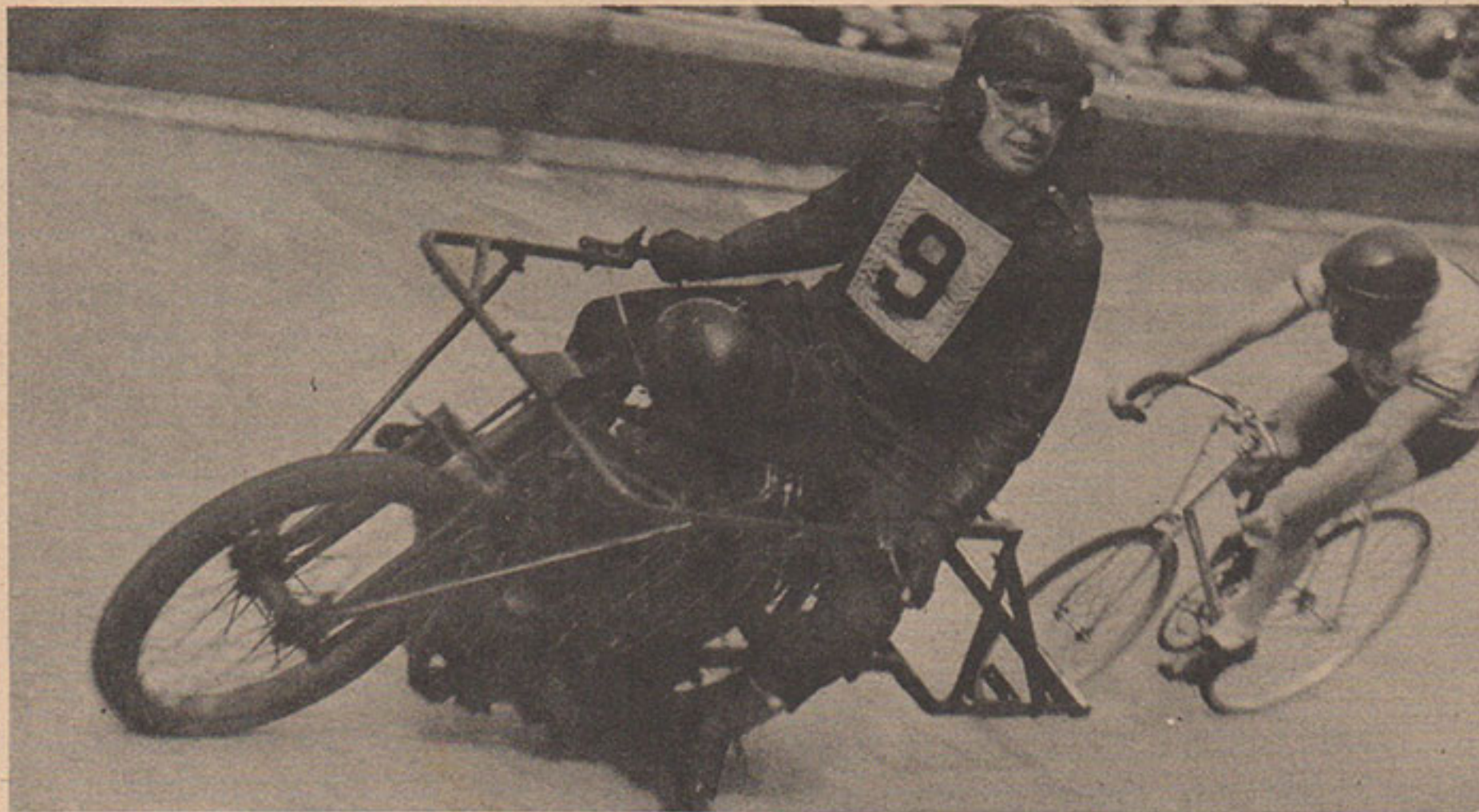
World Champion bicycle racer, Verschueren, of Belgium, hangs draft on an ancient pacing motorcycle. Bars are intentionally long to keep driver's arms at side for better wind-breaking
