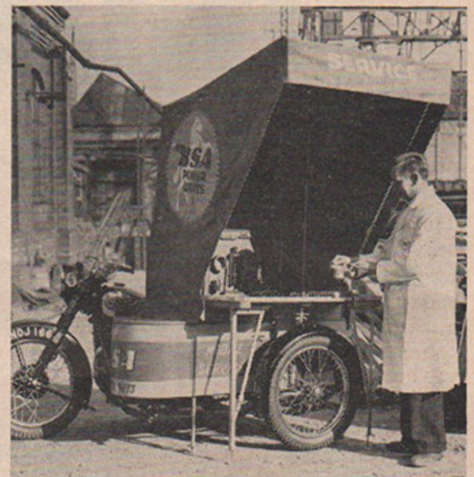
Compact and mobile sidecar-workbench carries all tools and spares necessary to service BSA powerplants. The range of BSA stationary power units has a wide variety of uses in agricultural and industrial equipment.
