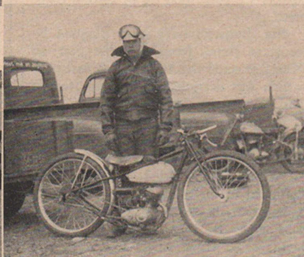
Built by H. J. Ottaway of Wichita, Kansas, this sanitary special is described as fastest 125 cc in the mid-west. Features a Whizzer tank, Servi-Cycle wheels and tires, a stock Harley-Davidson motor and carburetor, and a special frame and forks by Ottaway. Standing is Jerry Ottaway, 16.
