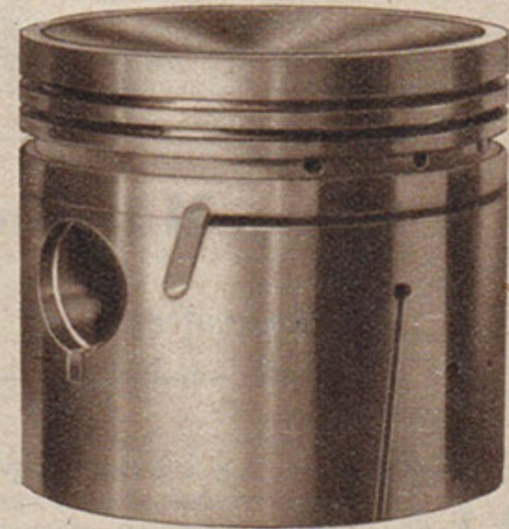
Special "flexible-skirt" piston employed with twin-cylinder engines. A10 engines have concave crown as shown; A7, flat crown
