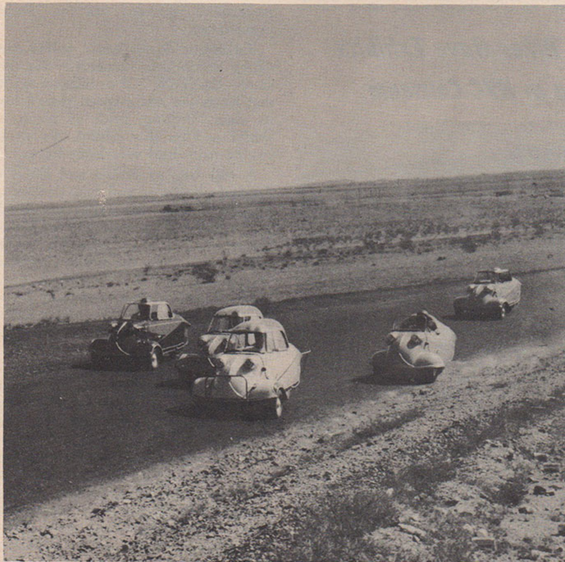
MESSERSCHMITTS: And then there was an egg-rolling contest. Messerschmitt cabin scooters put on a two-lap exhibition duel before bemused audience. Three-wheelers run 100 miles per gallon—have 197 cc engines.
