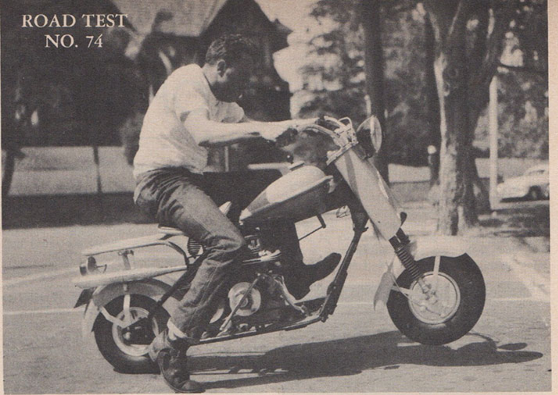
DRAG, CHIEF?: When you signal "full speed ahead" to the engine room of the Cushman Eagle, things happen. Five stout horses lifted front wheel and assistant editor Ron Britzke 'way high. Note starter ahead of engine, hand shift and foot clutch. Unphotogenic assistant editor adds little to otherwise-attractive decor of Eagle.
