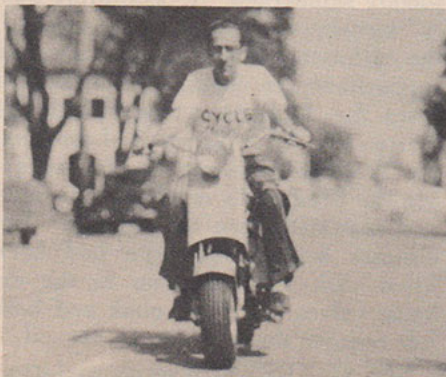
HEAD-ON: Enyeart presents photog with fine front view of attractive machine. Everything is accessible on this simply-constructed and easily maintained job. Footboards fold. Check rubber-mounted bars.
