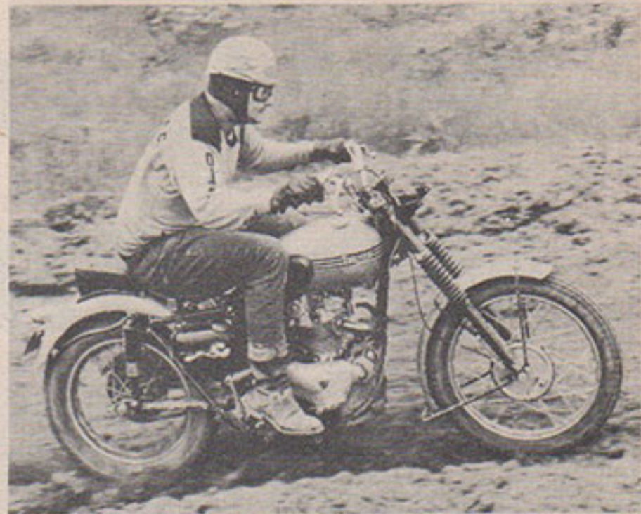
IN THE CHIPS: "Diz" Dizotell, the potato chip czar of Evansville, herds his Triumph over the muddy Indiana course. Note changes on TR 6—solo seat and pillion, PK Sportlight, Q. D. headlight removed and oddly enough, high bars in place of the usual flat handles.
