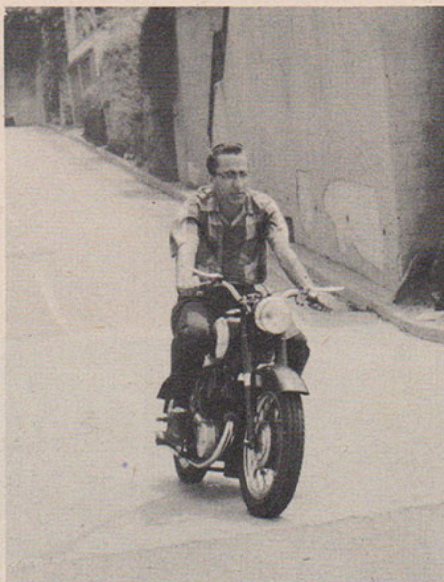
NO ECHO: Navy-bound Ron Enyeart motors quietly out of Echo Park road in Los Angeles. Twin exhausts and efficient mufflers kept Allstate's twin-piston, single-cylinder engine pleasingly silent. Enyeart, just learning to ride, will soon forsake civvies and test bikes for Navy garb.
