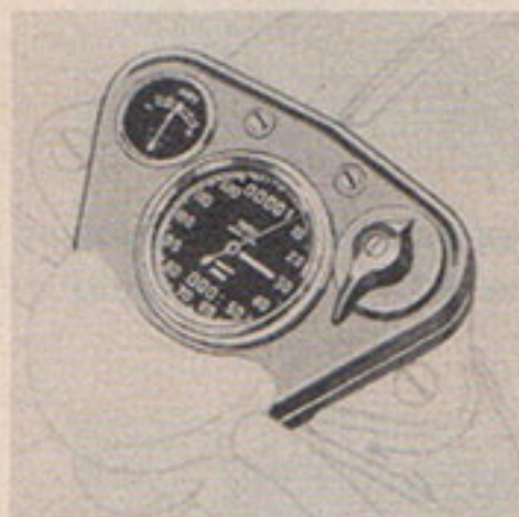
Ariel instrument panel groups. Speedometer, Ammeter, and lighting switch in neat style.
