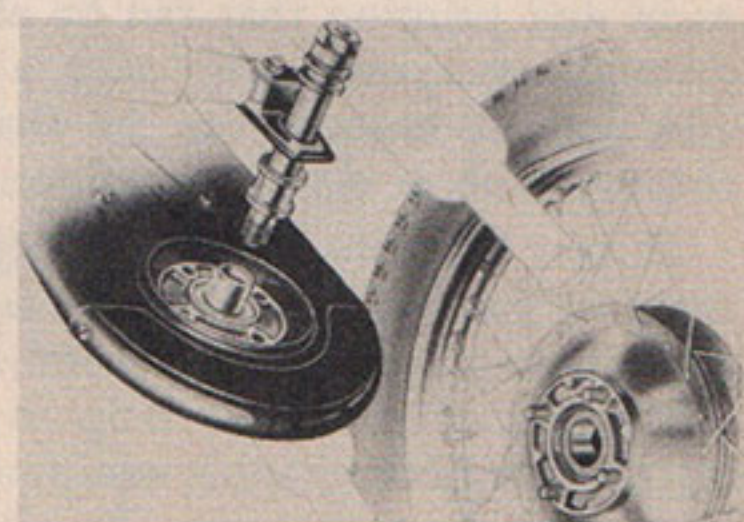
Quickly detachable rear wheel and rear chain enclosure on Ariel Huntmaster and Red Hunter models.
