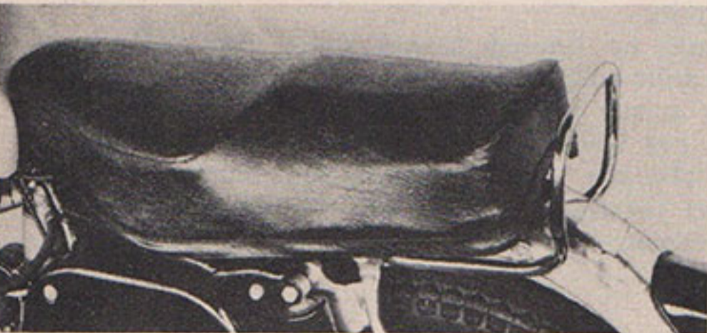
Wider, longer, and with softer foam rubber, here is the new "Twin-Solo" Dualseat specified for Eastern Models. Western models will have the trim "Cushionaire" Dualseat as shown on the model photos at right.
