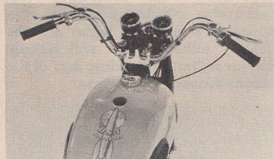
Standard equipment includes tachometer, steering head lock, steering dampner and manual spark advance.
