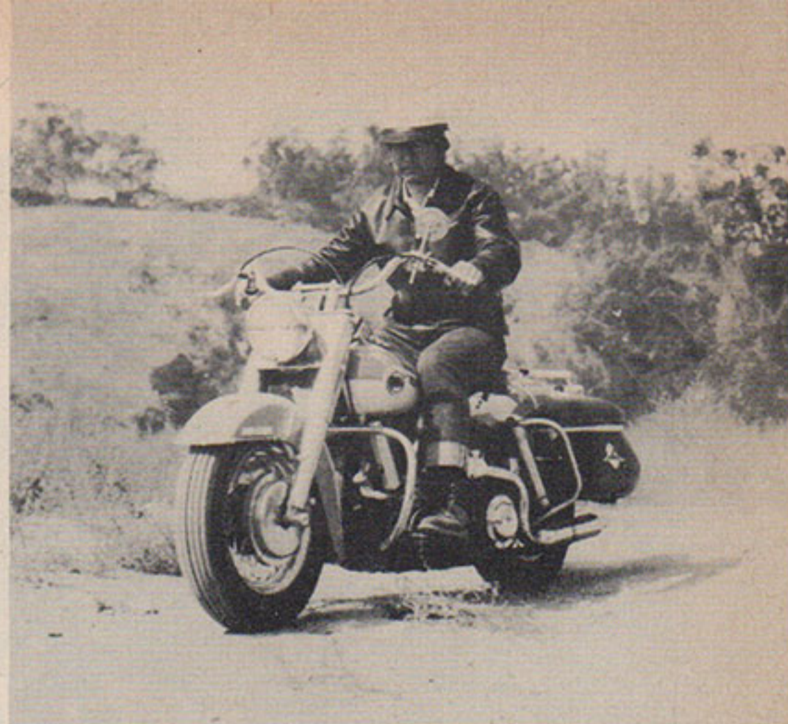
CRUISING WITHOUT BRUISING —The hydraulically-damped front and rear shocks made every road surface speedway-smooth, but forks rattled somewhat on rough trails.
