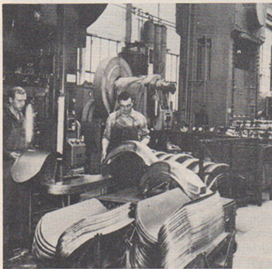
Fenders are made on these presses.
