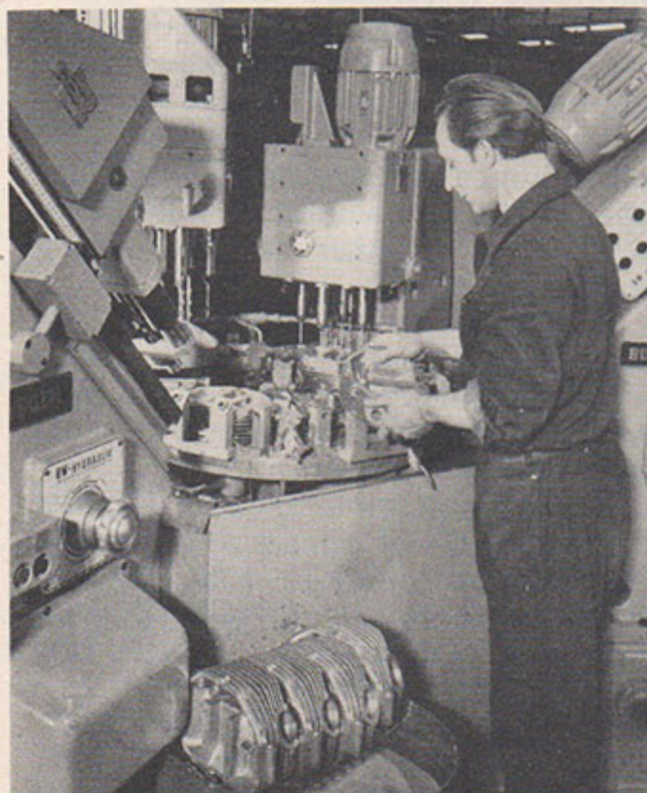
Cylinder heads are finished in one operation.
