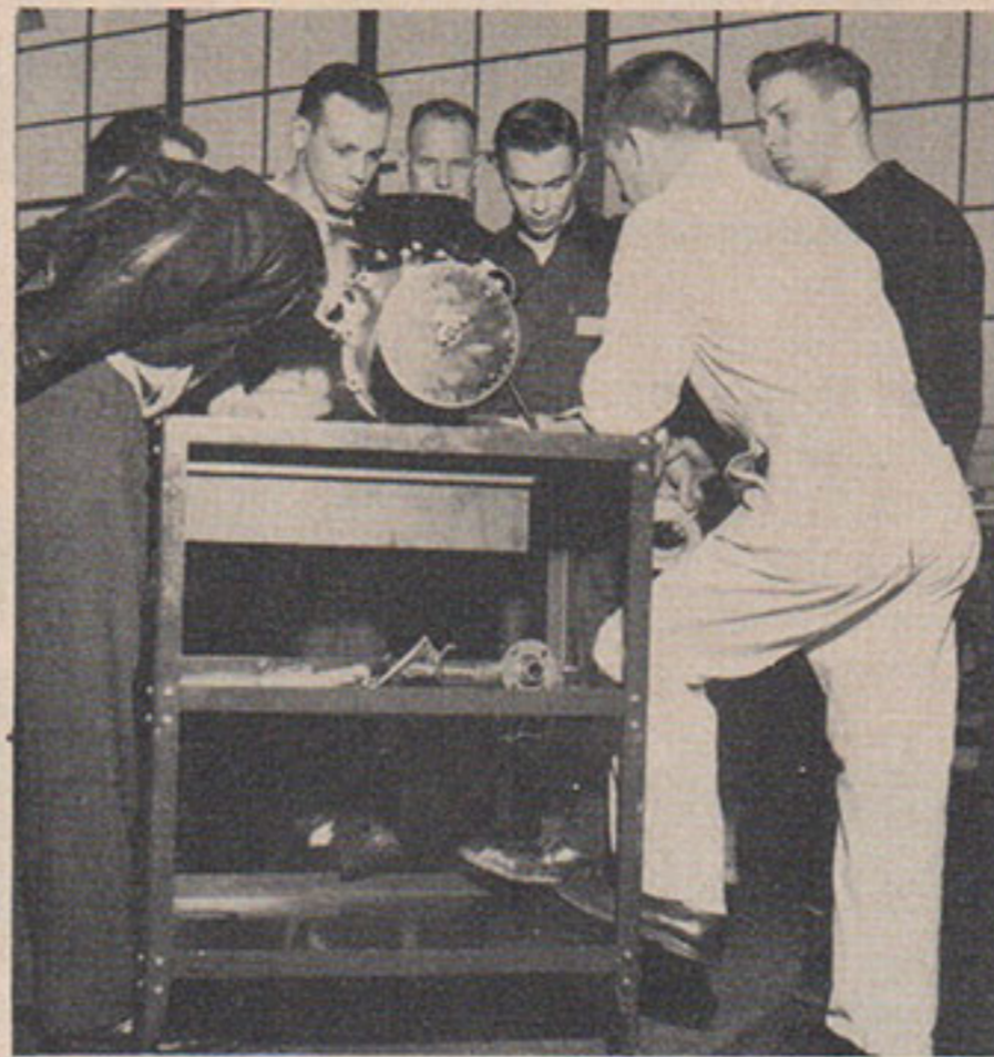
Service school instructor Cliff Guild shows some of his students the finer points of tuning a Triumph engine with a degree wheel.
