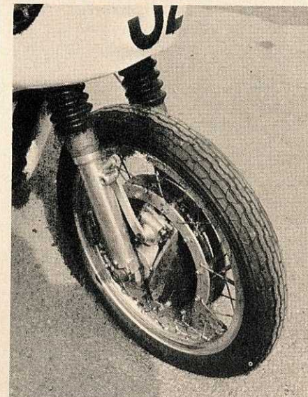
New brake idea employs a centrally-mounted disc with built up flanges to accept spokes.
