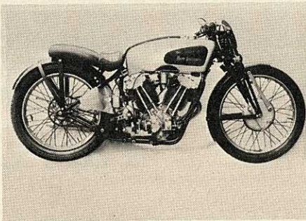
In 1934 New Imperial introduced this V-twin that turned 7500 rpm, ran 100 mph.
