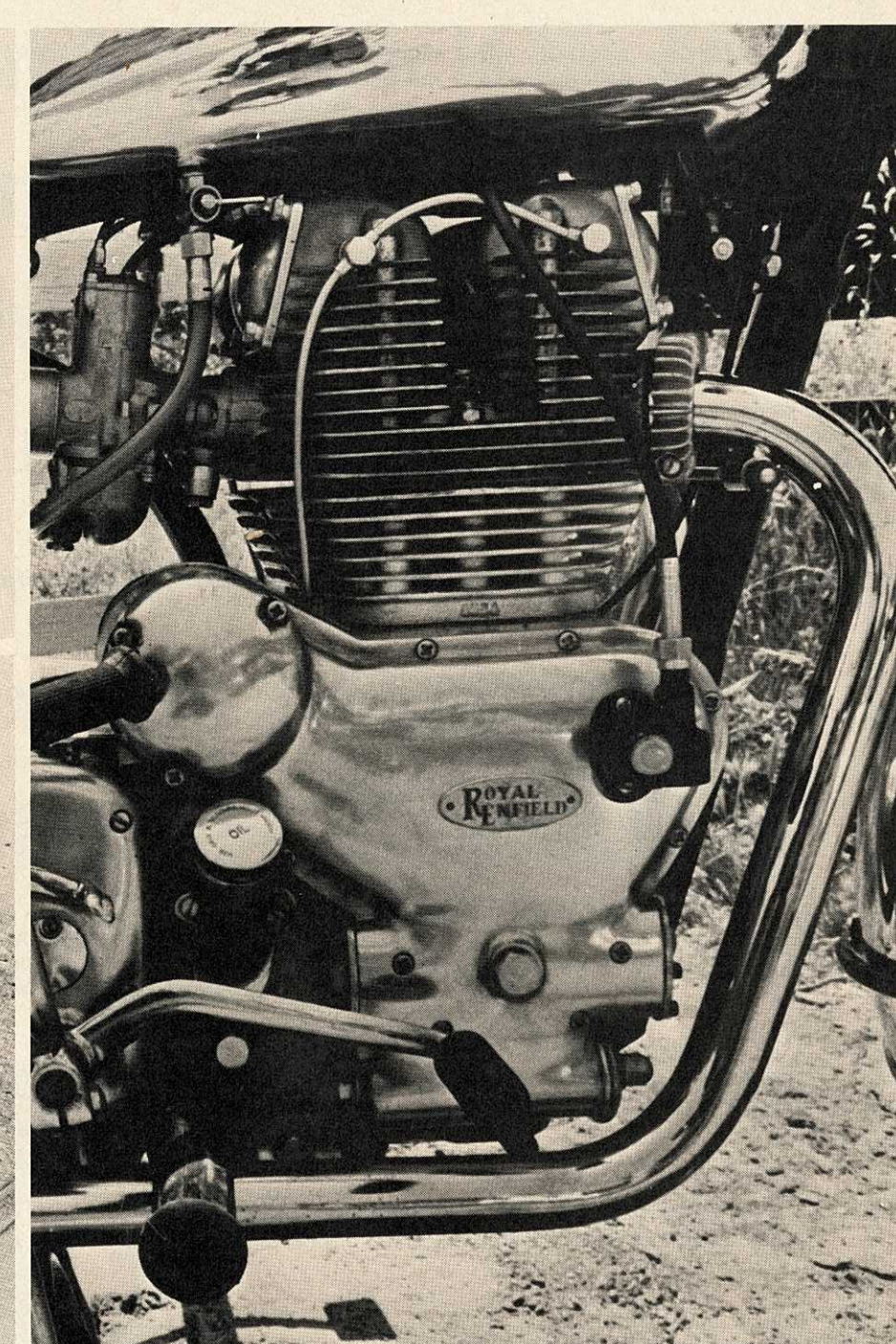
head houses rocker gear and provides for good cooling. Sturdy crank (above left) turns in roller bearings. Chrome-moly frame weighs only 26 pounds.
