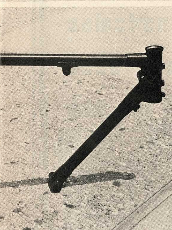
head houses rocker gear and provides for good cooling. Sturdy crank (above left) turns in roller bearings. Chrome-moly frame weighs only 26 pounds.
