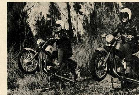
■ Doing "wheelies" isn't playing around. It helps to determine the handling characteristics and balance of the cycles tested.
