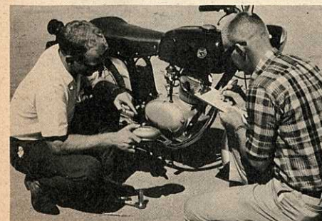
■ Air cleaner is removed at beginning of carburetor disassembly to see that it meets standard specifications.
