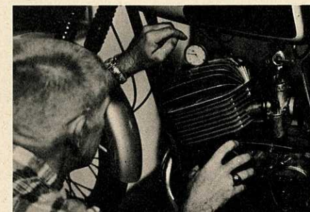
■ Finding top center on piston preparatory to timing ignition. Just one of the standard checks made on all equipment tested.
